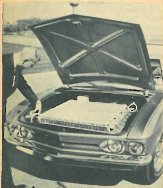
Electrovair II, by General Motors uses silver-zinc batteries for up to 80 miles of driving before recharge.
