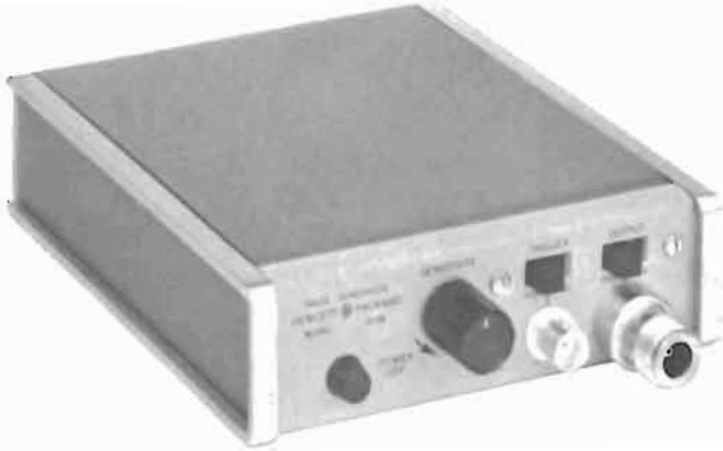
H-P 213B produces pulse with under 0.1-nanosecond rise time.
